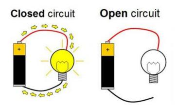
This same concept is used when using an on/off switch for a circuit. The "on" position produces a closed circuit and the "off" position provides an open circuit. The on/off switch is often symbolized with an icon (see icon image below). Similarly, the (a) diagram is switched on and the (b) diagram is switched off.
