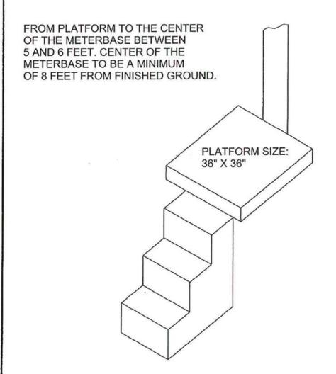
2' INCH TREATED WOOD, STEEL, OR CONCRETE MINIMUM
